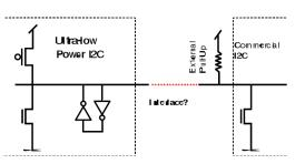
Figure 3: Two incompatible I2C implementations. Extreme care must be taken to not overpower the weak keeper. Driving signals to the low-power side requires manually driving the SDA line high both when writing and reading.
