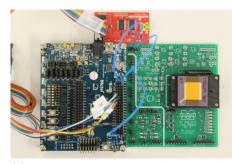
(a) The complete system: A commercial I2C device the BusPirate (top), the interface circuit realized in an IGLOO nano FPGA (left), and a breakout of the M3 control CPU board (right)
