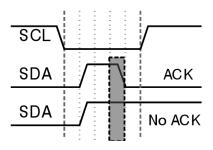
Figure 1: The ACK cycle of the modified I2C protocol. The negative clock edge is divided into 5 cycles: wait, pulse up, wait, pulse data, wait. These cycles are all 250ns long, permitting any clock rate up to 400kHz. The shaded region marks the only period in a I2C transaction the slave is responsible for driving.
