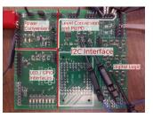
Figure 4: A combinational approach to interfacing the two divergent I2C systems. The M3 pull-up signal is supplied to a monostable multivibrator acting as a one-shot timer
