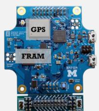
The Control Module provides non-volatile storage on an SD card and FRAM. It uses a GPS module to provide location and time data. The Control Module also manages and arbitrates power provided by the solar panel.
