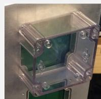
An off-the-shelf case seals modules to the waterproof sensing platform.
