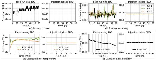
Figure 9: Stabilizing tunnel diode oscillators through injection locking phenomenon. Due to the trade-offs made to lower the power consumption of the TDO, it is unstable and prone to environmental changes (humidity, temperature). By injecting an external carrier signal into the TDO, the stability of the TDO is enhanced.
