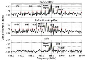
Figure 12: Comparison of spread of harmonics between backscatter and JUDO transmitter. JUDO transmitter does not generate unwanted harmonics because it allows the mixing of the analog baseband signal.
