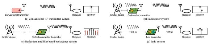
Figure 2: Comparing JUDO transmitter against transmitters commonly employed on WES. JUDO allows low-power transmissions while being spectral efficient. Unlike backscatter systems, JUDO allows the emitter device and receiver to be placed at considerable distances from the JUDO transmitter even at high bitrate (100 kbps). In contrast to reflection amplifiers based backscatter transmitters, it does not generate unwanted harmonics (harmonics are shown in red on the spectrum plot).
