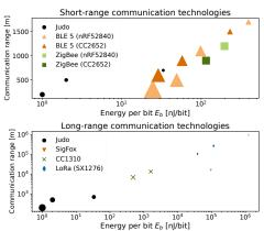
Figure 20: Comparing JUDO against commercial transmitters. The marker size represents the bitrate (min. 0.293 bps, max. 1 Mbps).
