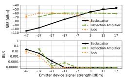
Figure 13: Signal strength and link reliability comparison between transmitters. This is done by varying the carrier strength of emitter device. Judo significantly outperforms the backscatter transmission when the carrier is weak.
